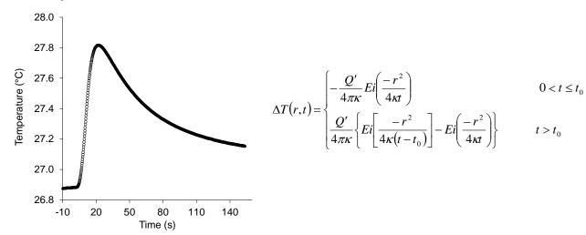
where t is time from beginning of heating, Q' is the source strength per unit time (m<sup>2</sup> K s<sup>-1</sup>),  $\kappa$  is the thermal diffusivity (m<sup>2</sup> s<sup>-1</sup>) of the medium surrounding the heater, and -Ei(-x) is the exponential integral function with argument x. Q' is defined as  $Q' = q'/\rho c$ , where q' is the energy input per unit length of heater per unit time (W m<sup>-1</sup>) and  $\rho c$  is the volumetric heat capacity (J m<sup>-3</sup> K<sup>-1</sup>).
