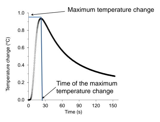
where  $r_n$  is the needle spacing of the DPHP (m),  $t_m$  is the time of the maximum temperature change (s), and  $\Delta T_m$  is the maximum temperature increase (K) as recorded from the DPHP thermistor.
