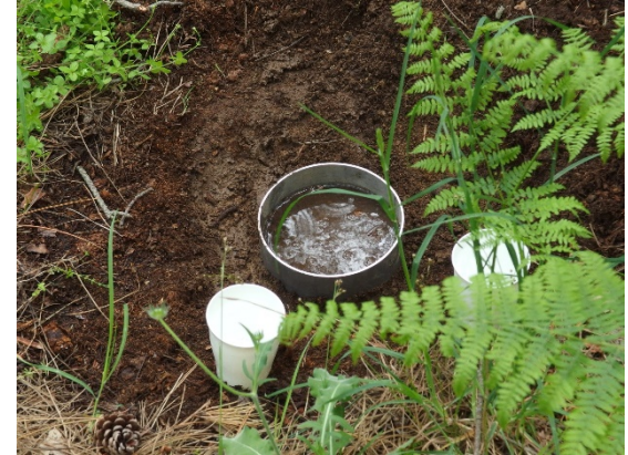
3 Register the infiltration time
