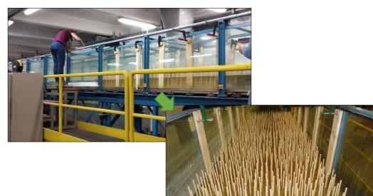
Vegetation (Dowels): Diameters: 8mm and 4mm Height of cylinder: 0.30m Longitude vegetation: 5.0m, Material: Balsa and Ayous
