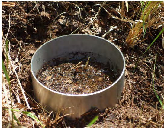
4 Measurement of the soil water content at the end of the measurements
