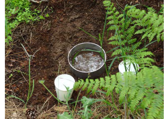
3 Register the infiltration time
