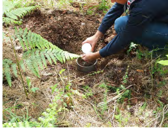
4 Measurement of the soil water content at the end of the measurements
