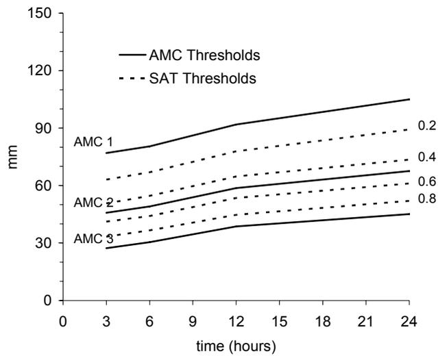
**Fig. 1** Rainfall thresholds computed for the Rignano cross-section, on the River Arno, Italy. Solid lines show thresholds estimated for the three levels of AMC following classical SCS-CN guidelines. Dotted lines show thresholds estimated according to the alternative approach as a function of the 0.2, 0.4, 0.6, 0.8 soil degree of saturation.
