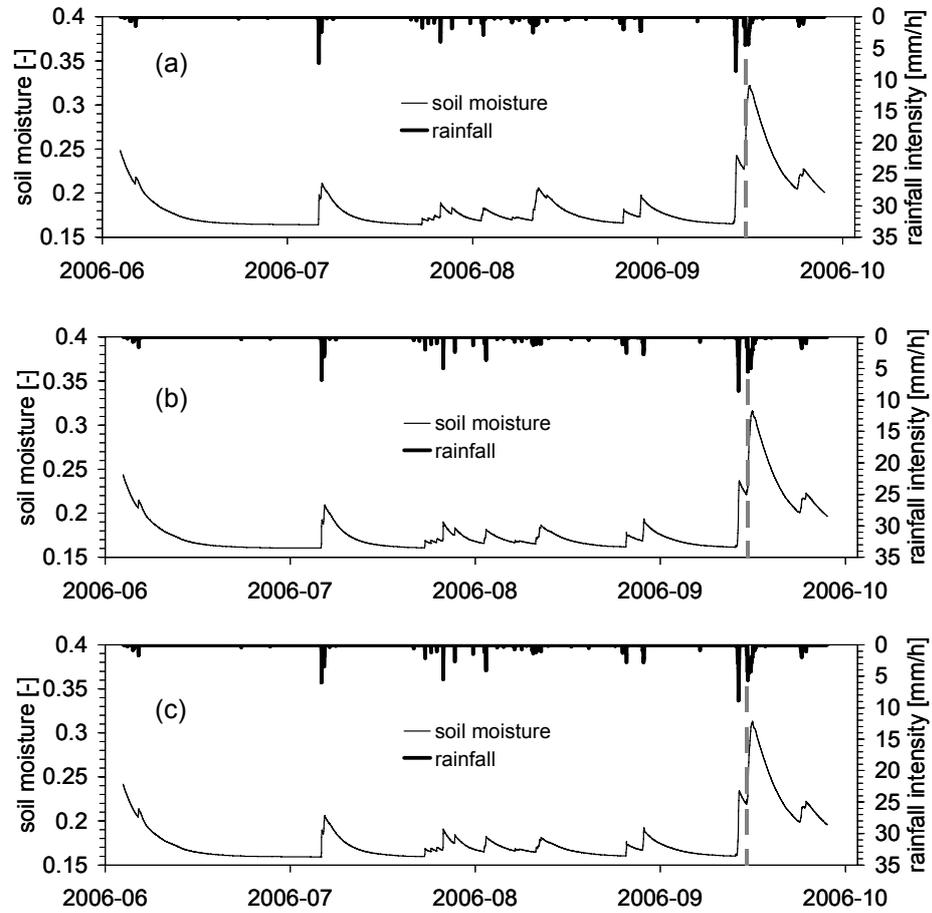
**Fig. 4** Soil moisture dynamic (thin black line) simulated by means of FEST for the sub-basins of Nave di Rosano (a), Rignano (b), and S. Giovanni Valdarno (c). Vertical dotted grey line points out the beginning of the event.
