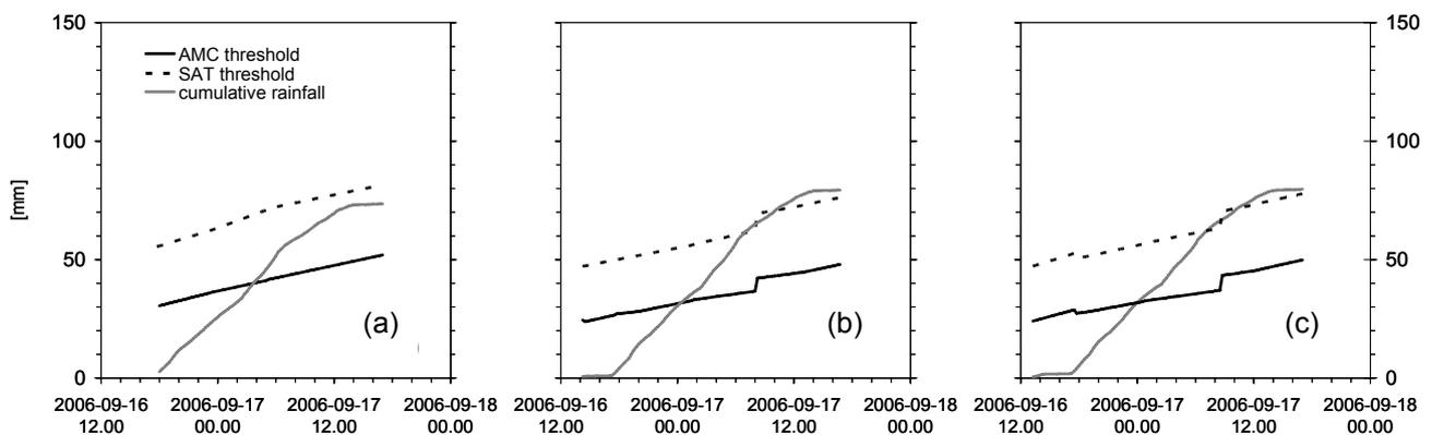
**Fig. 3** Results of the monitoring of the 17 September 2006 flood event at the sections: Nave di Rosano (a), Rignano (b), S. Giovanni Valdarno (c). Cumulated rainfall (solid grey line) is compared to AMC threshold (solid black line) and SAT threshold (dotted black line).
