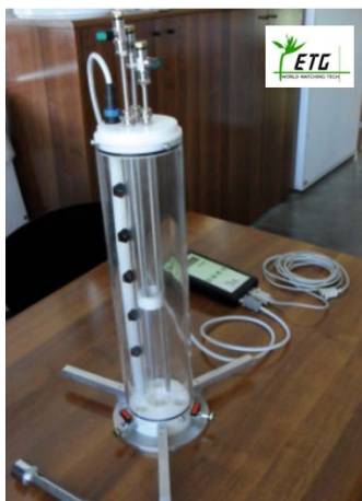
Figure 2. The portable calibrator (a) and field verification results for the three raingauges operating at a resolution of one minute (b).
